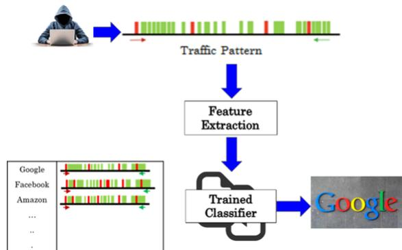
Figure 3: Feeding Traffic Pattern into Trained Machine Learning Classifier.
