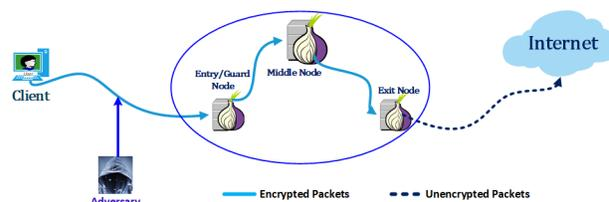
Figure 1: Website Fingerprinting Attack Model.
